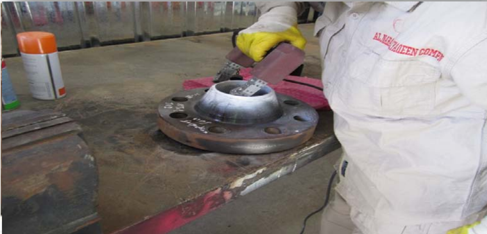
Magnetic Test Tools And Spray Sets For Inspection Defects On Piping And Structure Work
